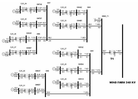
Figure 2 (b): T1 Collector Circuit
